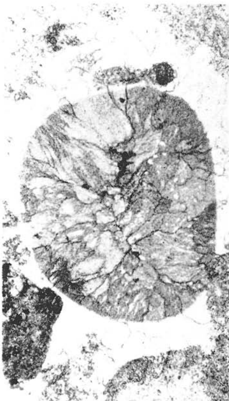
Fig. 7. Dedolomite of the type B. Phantoms of the original pebble are visible due to brown pigmentation. The filling consists mostly of elongated calcite individuals of radial orientation. H. Vadičov — a. Thin section No. 10016. Magn. 48\times .
